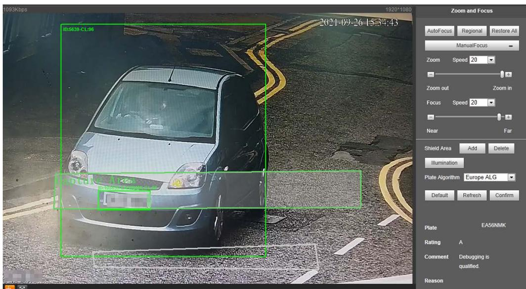
**Step 2** Set the focus and zoom mode, which is used to recognize vehicle.
