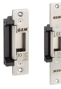
This ANSI style release offers flexibility, being supplied with both long and short face plates, and is field selectable for 12V or 24V power, and fail-safe or fail-secure operation.
