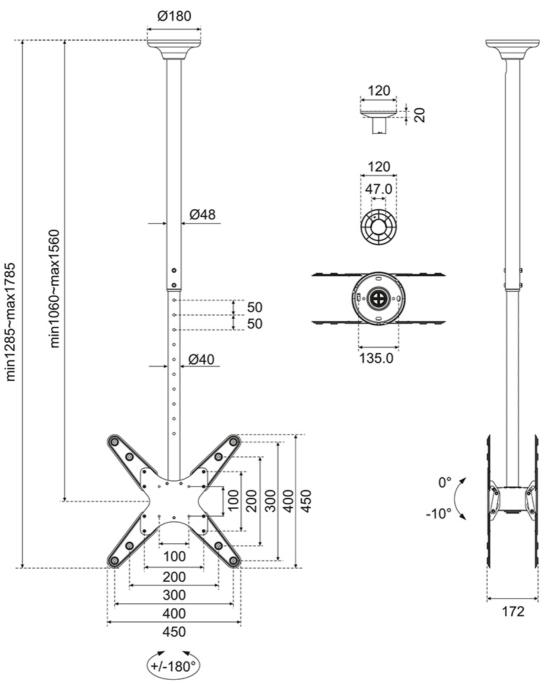
Neomounts Measuring unit: mm
