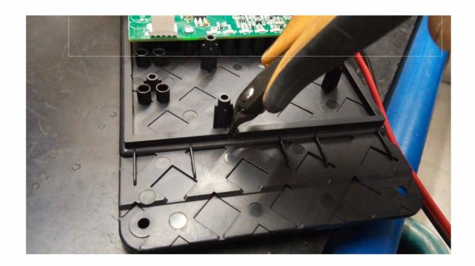
Practice a second cut as in the picture and then use a cutter to smooth the hole created.
