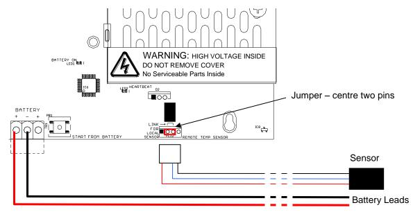
NOTE: If the base card is not fitted with either a jumper or a remote temperature sensor the panel will indicate a charger failure condition. Ensure that the jumper is replaced if the remote sensor is removed / not used.
