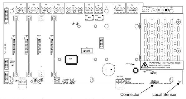
To install the Mxp-501, first remove the jumper link from the connector.
