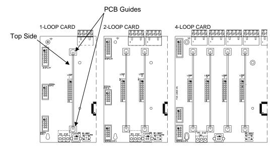
Insert the Loop Driver PCB so that the top side is oriented to the left as shown.
