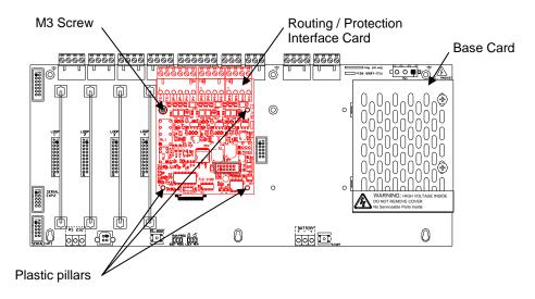
To remove a routing / protection interface card:
