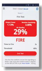
Press Start Test to perform a fire test, this works by running a test algorithm to lower the output power, the receiver sees this as obscuration.
