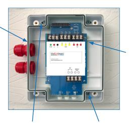
Screw in through holes provided outside of the rubber seal
