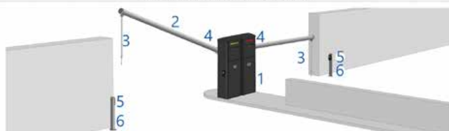
COD. 649261 Art. BOOM6 DEA round painted boom 6125xØ60mm, with reflective red stickers art. 1012
